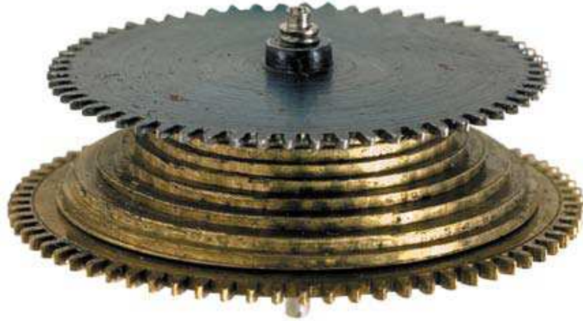
Picture 6: The fusee including all what has been seen above
